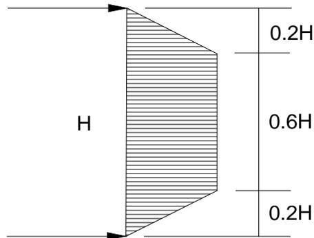
7.18.19 It is very important to note that active pressures can only be achieved when movement in the soil (earth wall) occurs. If movement in the soil is not acceptable, such as adjacent to an existing structure, an at-rest pressure of 45 and 59 pcf should be considered for the design of 12 foot and 25 foot high shoring, respectively.
